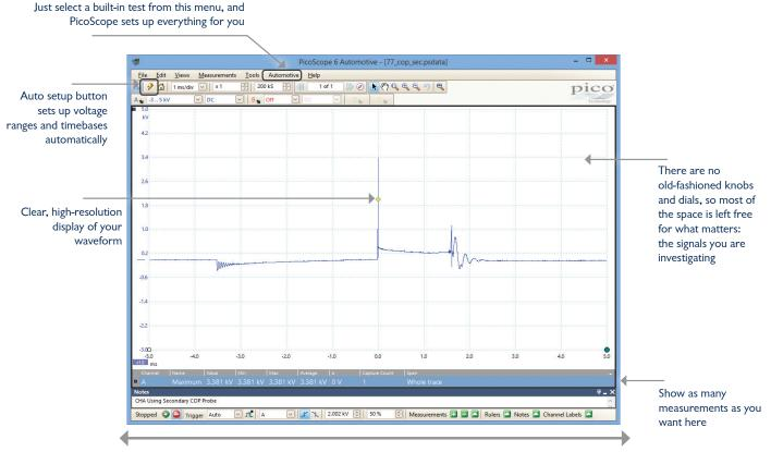
Because PicoScope runs on your PC, it can use the whole width of the computer screen. The display size is not limited by the size of the scope.
