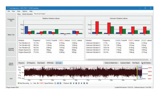
On the analysis page you can move the bar within the signal history chart (at the bottom of the screen), to view portions of time and look for changes in vibration orders and high levels of frequency changes. These spikes indicate the component type that is likely to cause the issue. The information provided by PicoDiagnostics is very clear and detailed, complete with a help system to guide you through your results and the likely causes to investigate.
