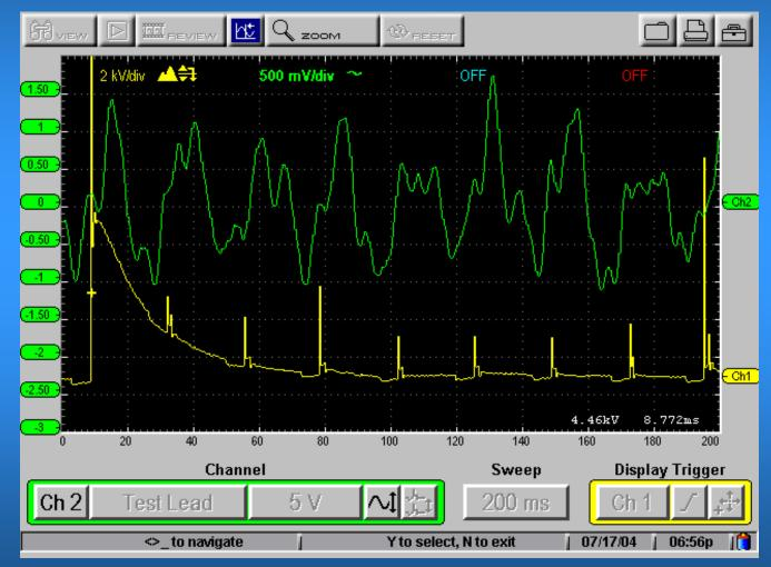
The time between #1 cylinder ignition triggers is 186.30ms
