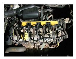
This system can only be tested if you have the same number of extension leads as coils within the cartridge coil-pack. The cartridge coil-pack is fitted directly over all the spark plugs and lifts off in one unit.
